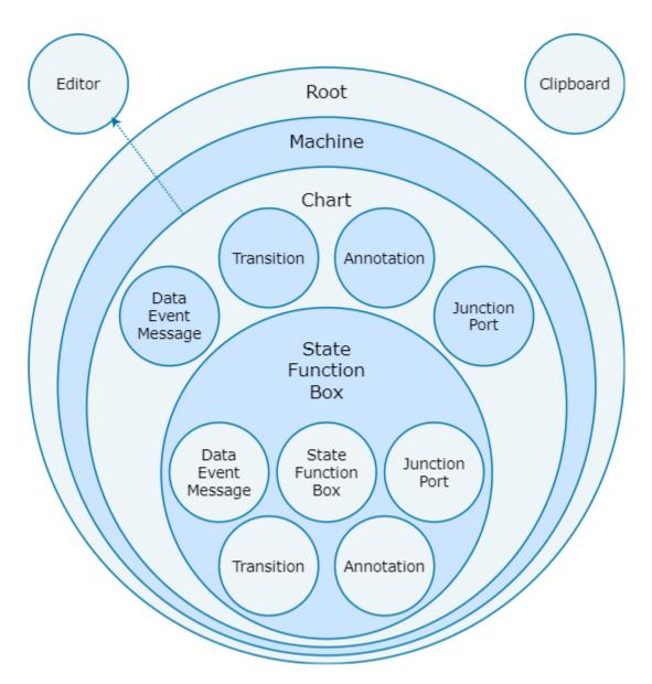
The hierarchy consists of four levels of containment:
