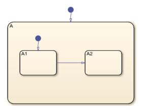
Calling the find function to find all the states in this chart returns an array with three Stateflow. State objects:
